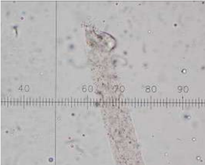
Fig 4. This polyester fiber, seen in plane polarized light, was cut with a scissor.
