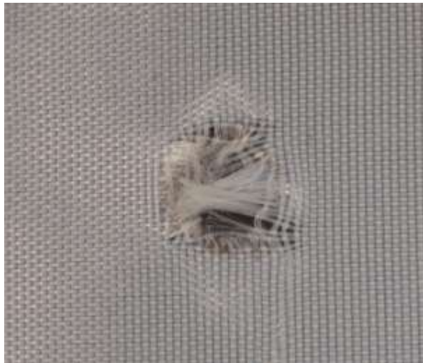
Fig 3. A polyester fabric that was shot with a 9 mm full metal jacketed bullet, with a velocity of 1150 feet per second
