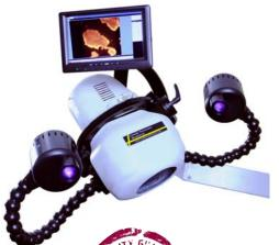
The LSV Advantage: With its freely rotating gimble system, containing over 59" of horizontal reach and 40" of vertical height adjustment, the LSV has a massive reach and spread allowing it to effortlessly cover evidence tables.
