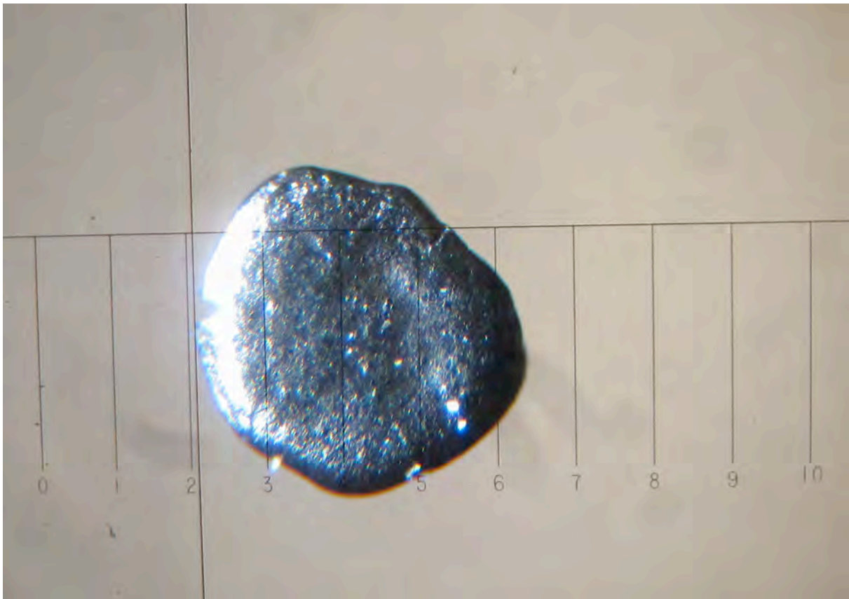
Image of smokeless powder particle viewed through microscope equipped with filar reticle. Note position of the long vertical line “touching” the left edge of the particle
