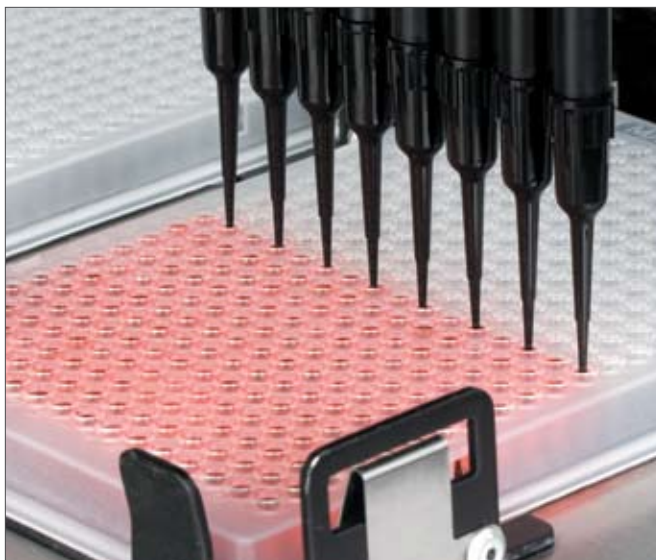
Figure 2. The JANUS Varispan arm (8-tip shown), provides the flexibility and pipetting precision needed for full forensic application processing from DNA purification and normalization to PCR master mix creation and PCR setup.
