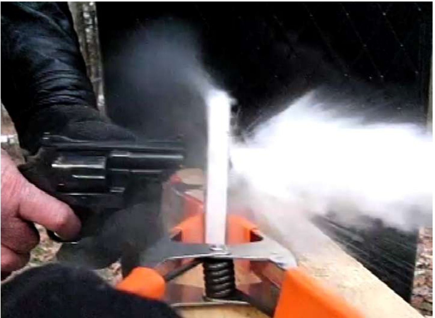
Photo: 38 Special at the moment of discharge to another piece of 1/2" gypsum wallboard, in this instance orthogonal to the surface.
